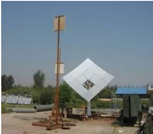
High order surface heliostat
