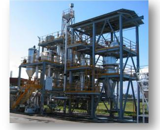
The Circulating Fluidised Bed steam-gasification Reactor coupled with Molten Carbonate Fuel Cell
