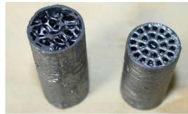
Engineered cellular SiC tubes from SUPSI and Yeungnam University tested for solar gas turbine application
