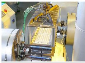
10 kWh plate heat exchanger test setup
