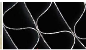
Corrugated metal foil structures from EMITEC tested for volumetric receiver application
