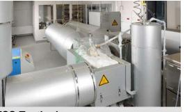
**TCS-Testbed** Thermochemical storage test facility for temperatures up to 1000 °C
