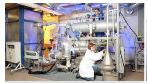
Skoop Latent heat storage test facility for temperatures up to 400 °C
