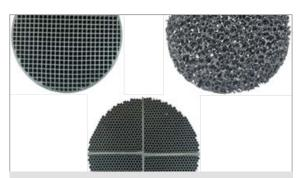
Volumetric absorber structures
