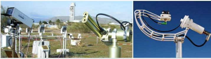
Equipment for sunshape measurement: Visidyne's SAM (left) and CIMEL sunphotometer (right) at the Plataforma Solar de Almería
