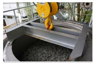
Inner chamber of testbed with storage material
