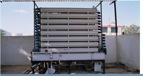
This project aims to evaluate the thermal performance of vacuum tube solar collectors to provide MSF desalination unit with continues hot water at 80 °C
