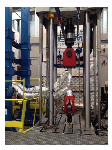
Insert Fatigue Test at Constant Temperature (Maximum Load 1 MNI)
