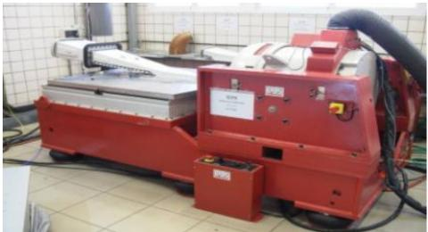
Vibration Test System V875-HBT 640
