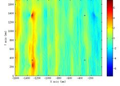
Slope Deviations of RP3 innerFacet Mirror by 2-Projector System [mrad] (positive = normal Vector is tilted in negative x-Direction)
