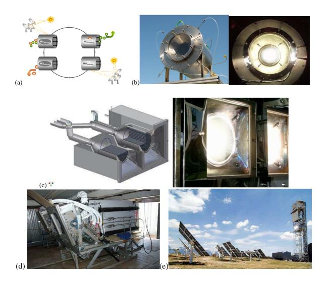
**Figure 30** Solar reactors employing honeycombs; the HYDROSOL reactor technology evolution: (a) operating concept; (b) first single-chamber reactor assembled and in operation; (c) the continuous solar hydrogen production operation concept and the first dual-chamber reactor in operation; (d) the 100 kW-scale dual-chamber reactor on the top of the PSA solar tower; (e) operation of the reactor coupled with the solar field.
