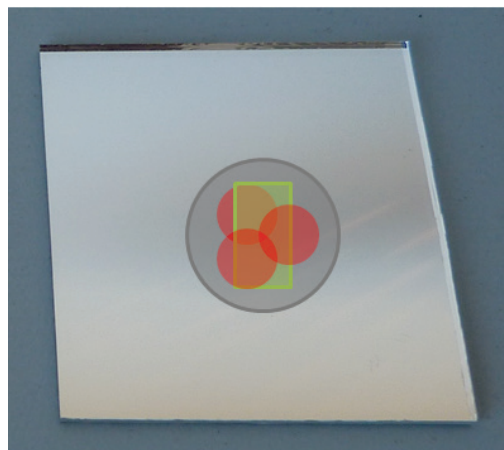
Fig. 1: illustration of the positioning of the measurement spots on a reflector sample. The grey circle represents the minimum area of the erosion experiment (2.5 cm diameter), the red circles stand for the D&S measurement spots (1 cm diameter with allowed overlap) and the green rectangle for the measurement spot of a Lambda 1050 spectrophotometer from Perkin Elmer (17 x 9 mm 2 ) in the 0° measurement position. This spot shall be rotated two times by 90°.
