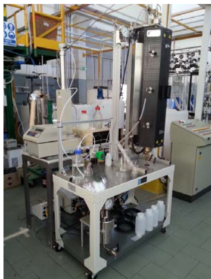
Figure 10. Facility for biomass gasification at ENEA Trisaia laboratory
