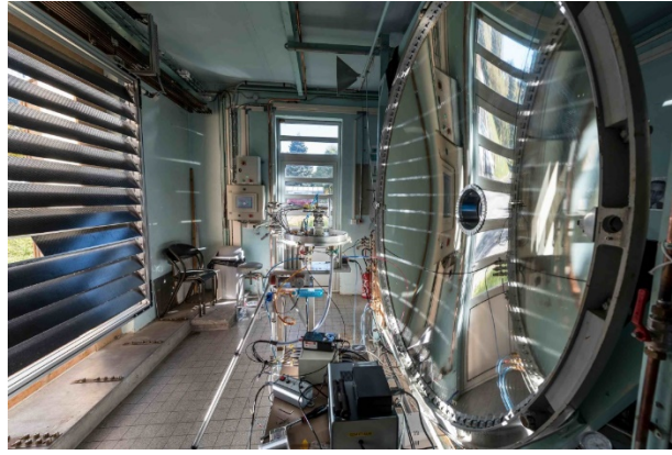
Figure 30. The DISCO setup. An optical fibre emits a solar beam perpendicular to the surface of the sample placed at the focus of a solar furnace, while eight fibres collect the reflected flux in different directions, from 0° to 70°.
