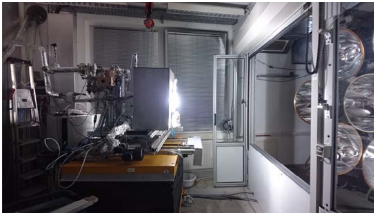
Figure 36: Solar receiver operating in the solar simulator at DLR, Cologne.
